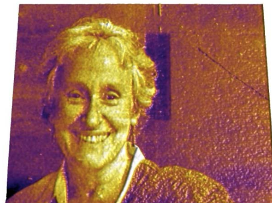
1 micron x 1 micron sculpture of Jane in silicon oxide. Z-scale = 2nm. Created at Asylum Research by Ted Limpoco using an AFM operating in anodic oxidation mode on the surface of a silicon wafer. Presented to Jane by Roger Proksch of Asylum Research on the occasion of her receiving the 2017 ACS Industrial Chemist Award.
