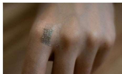
Images of stretchable organic transistors. Image credit: Amir Foudeh, Jie Xu, Sihong Liu of Bao Group, Stanford University
